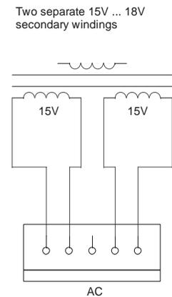
primary / mains voltage side not shown. Only work with mains voltage when you are qualified - then you know how to connect fuses, switches, earth GND etc. as well. If not, let some qualified person do it, or use a wall wart instead.
